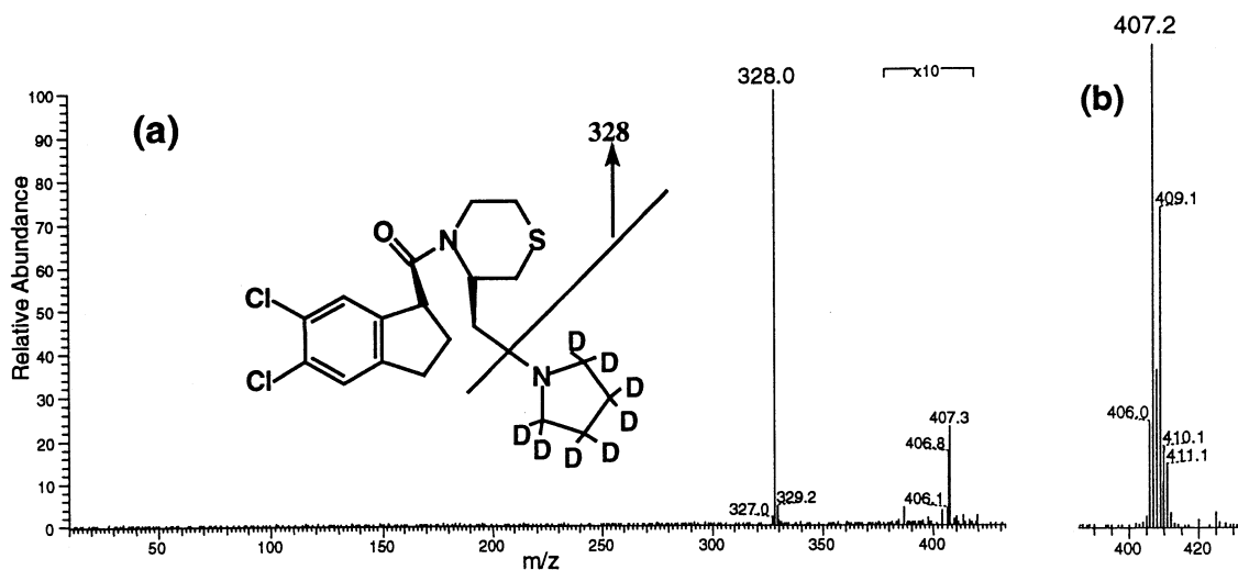
Fig. 2. ESI-MS, ESI-MS/MS spectra of d_8 -R-84760 (50 ng/inj): (a) ESI-MS/MS spectrum of d_8 -R-84760 ( m/z 407) and its fragment pattern; (b) part of ESI-MS spectrum of d_8 -R-84760.
